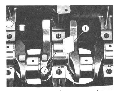
When checking and replacement procedures have been carried out, install caps and tighten bolts to 59 ft. lbs. (8.2 kgm) torque.
