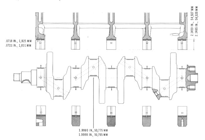
When regrinding journals, be sure to pay special attention to specified fit clearances in relationship to undersize bearing range available for service. Depending on amount of wear, main bearing journals and crankpins should be reground to undersize diameter shown in tables.
