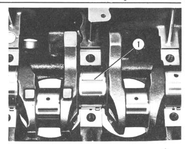
Install caps, complete with bearing shells. Tighten cap mounting screws to a torque of 59 ft. lbs. (8.2 kgm).
