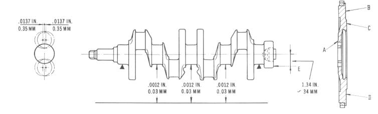
Maximum allowable misalignment of journals and crankpins, and diagram for checking flywheel contact surfaces with clutch disc and crankshaft flange.
