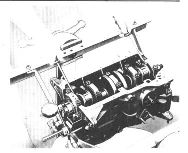
Should end play prove to be more than maximum allowable limit of .0137 in. (0.35 mm), replace thrust rings with .005 in. (0.127 mm) oversize rings.
