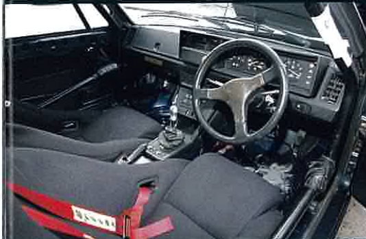
Interior's been stripped-out to achieve a lightweight 830 kg.
