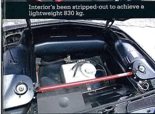
Strut brace and aluminium fuel tank take residence in the front.
