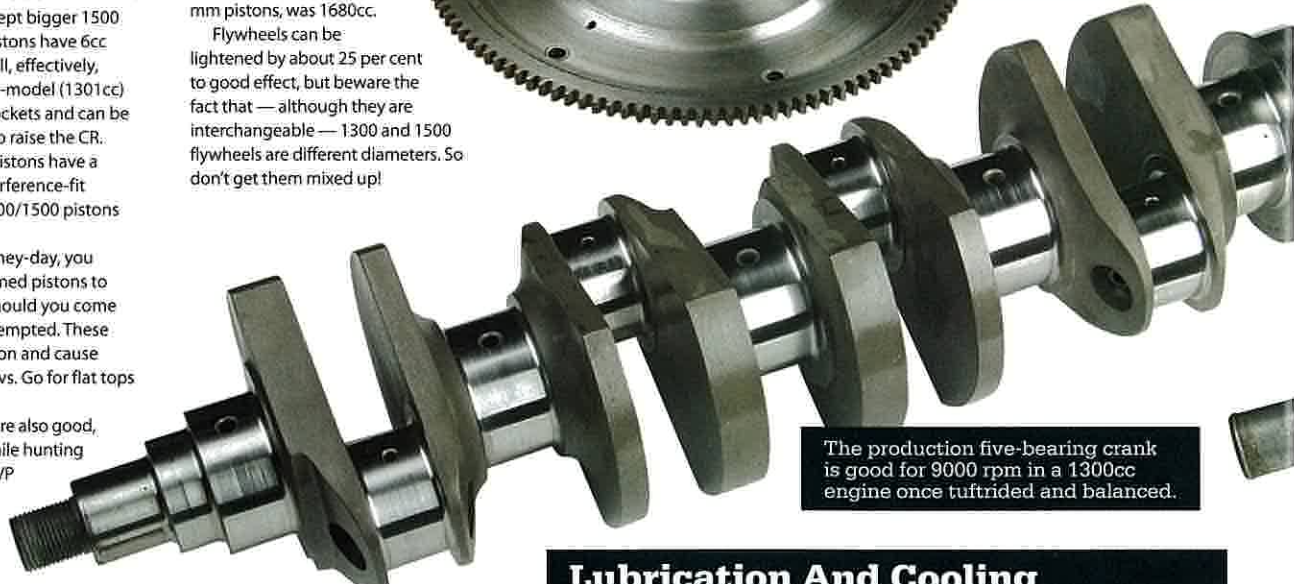
The stock flywheel can be lightened. The 1300 and 1500 engines are different diameters.
