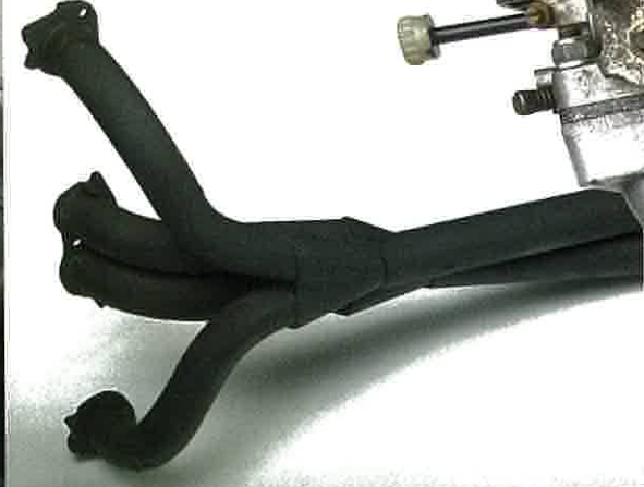
The production cast iron exhaust manifold is not too bad — but four-branch improves gasflow.
