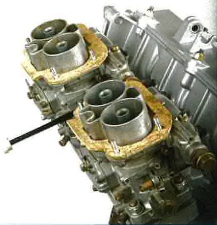
Dual Weber DCF carbs are the ones that fit within the X1/9 and 128 engine bays without the need for panelbashing.
