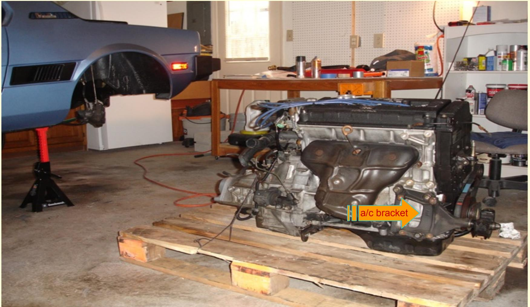
In this photo I've already removed the intake manifold and its support bracket to allow the motor to fit in the car. Hopefully I can figure out where all of these hoses and wires go. Remember to tape over the intake ports and other openings to prevent any foreign objects/dirt from getting into the engine or transmission.
