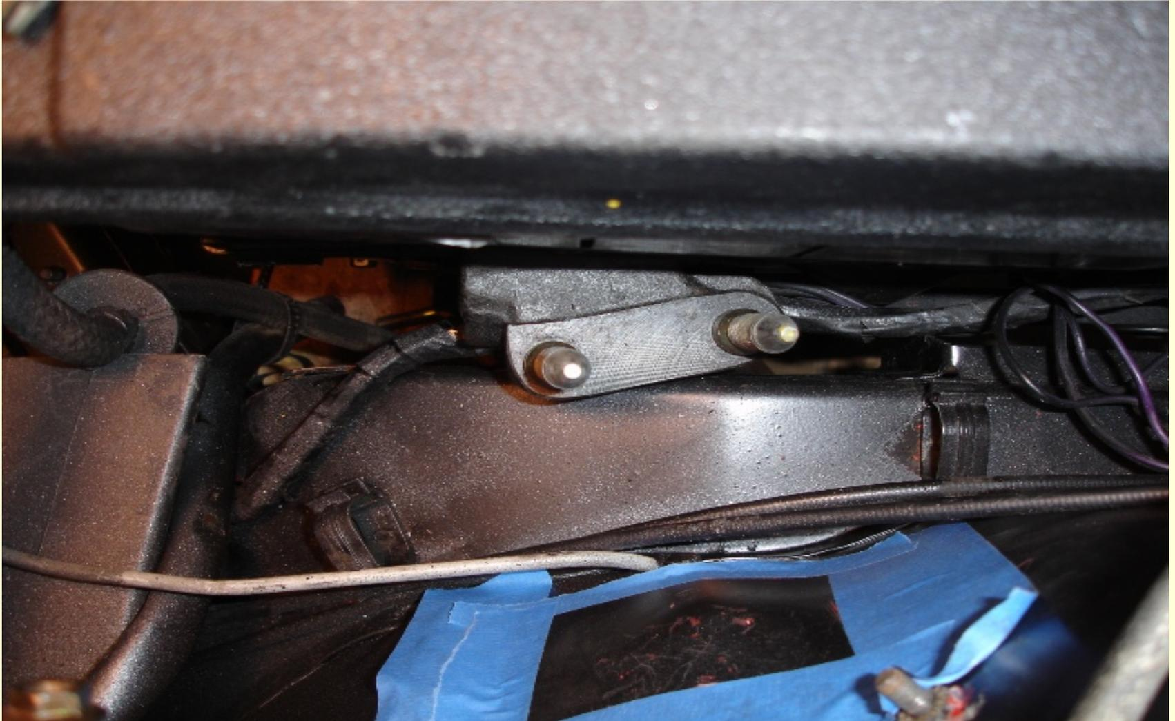
This photo shows my torque mount and transmission mount, both professionally welded together after I cut them to size. I didn't want to trust my beginner's welding skills on something this critical. I'll stick to welding things like the shift lever and shift rods. Notice the gussets added to the tranny mount for additional strength.
