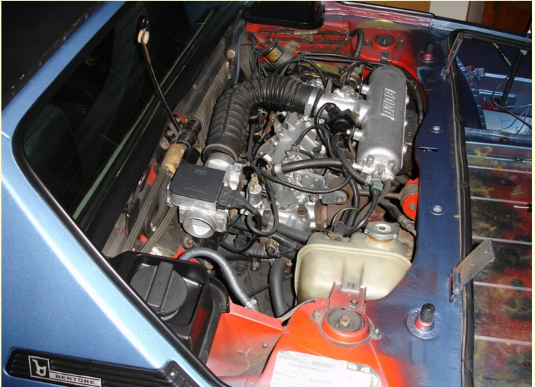
It didn't take that long to pull the motor and tranny as I wasn't too worried about breaking things. While waiting for the B16 to arrive I cleaned up the bay and repainted it. Note that I kept the starter wires, throttle link cable, heater hoses, back-up light connections. I'll need those later. The only wires I removed initially were the wires from the ecu to the engine. Later, I removed the wires to the fuel pump and the old ignition wires.
