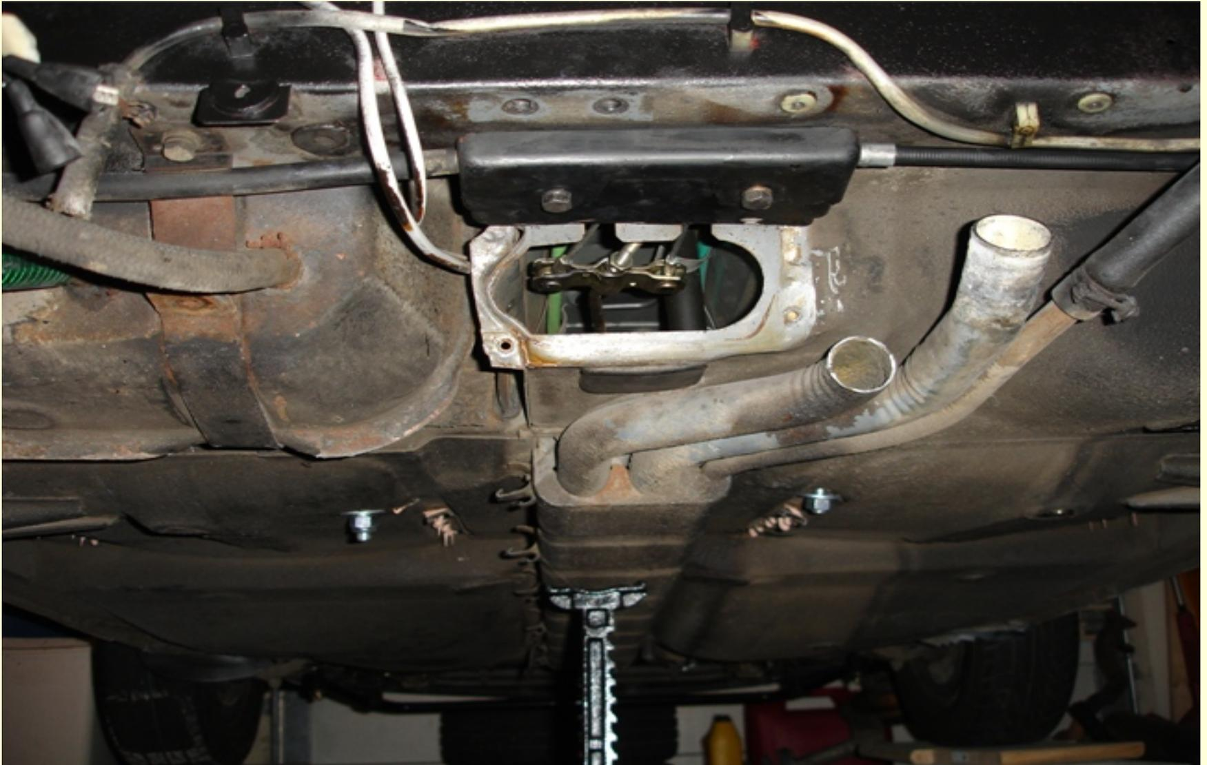
With the engine still out of the car, I cut some notches in the lip of the right (passenger side) inner fender guard and bend the lip outwards. This allows the end of the Honda transmission to be slid in close to the slanted edge which helps to get the drive shafts into proper alignment.. Note: this is not the final position of the transmission.
