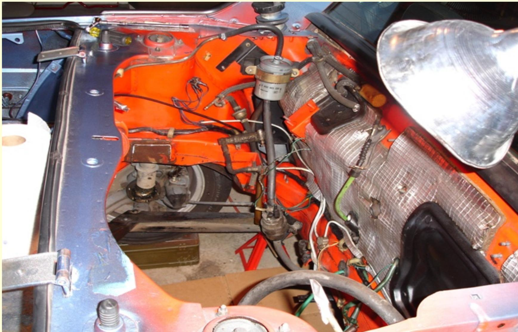
Now was the perfect time to clean and paint the engine bay. I tried various degreasers and found that acetone seemed to work best. Acetone eats into paint so I wouldn't recommend using it unless you plan to repaint the bay. I also lightly sprayed the firewall insulation with high temp bright silver paint after I cleaned it.
