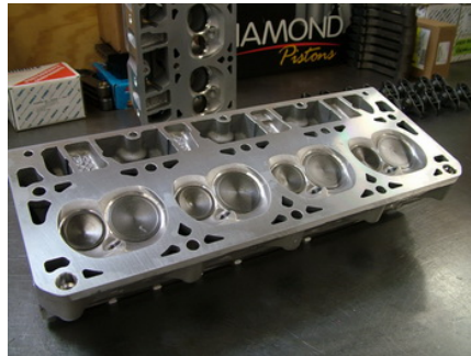
Coolant passages in the cylinder head.
