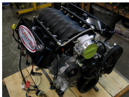
Overall shot of my LS2 showing all the coolant inlets and outlets.
