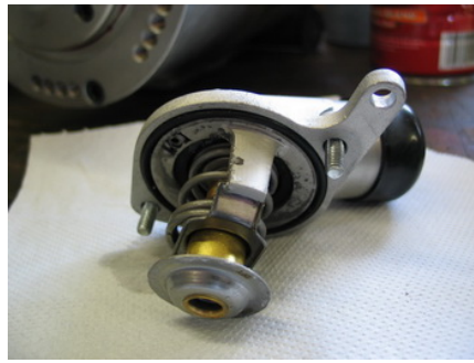
LS1 thermostat located in the integral thermostat / pump inlet housing. This particular thermostat is rated at 180°F.
