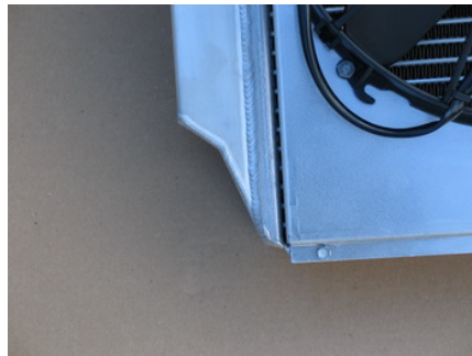
Custom notch to clear tubular frame rails.
