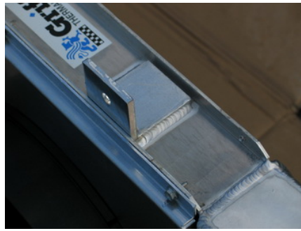
Aluminum mounting bracket welded to upper channel.
