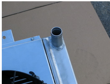
1.25" radiator inlet on upper right tank.
