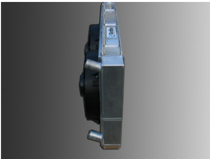
Side view. The rad is 3" thick. With the shroud and fans it is a total of 7.76" thick.
