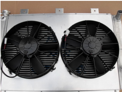
The fans are twin 305mm (12") SPAL VA01 - AP70/LL - 36A electric axial motor paddle-blade high-performance individually balanced units with sealed waterproof motors. The complete spec sheet for the fans reveal that, combined, they pull 3280 CFM.
