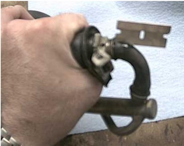
Be very careful to minimize scoring the barbs. This is where the sealing occurs and any deep scoring caused by the knife can lead to leaks.
