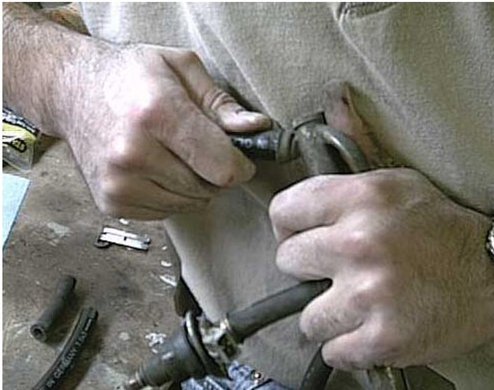
Use the old piece of hose to size the new one. I always add another .060" of length to account for any shrinkage of the original hose. Make sure the cut is as clean and straight as possible. I first install the hose on the rail. When installing the new hose, push it firmly against the collar as hard as you can. Be sure that the outer diameter of the hose has in fact squeezed itself entirely inside the collar. It is this compression of the hose inside the collar that helps the sealing process.
