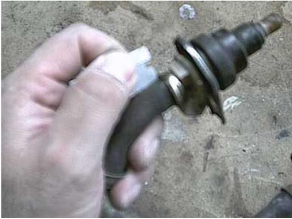
The hardest part of the procedure is removing the old hose from the barbs. I've found that the best tool for the job is a nice sharp exacto knife or a fresh razor blade. The trick is to cut the hose as far under the collar as possible. You want to cut it along it's length.
