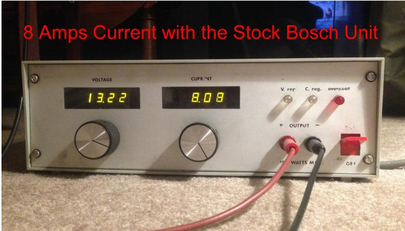
The new HEI / Bosch unit drew only 3.8 Amps under the same condition. A 4.2 amp savings and a cooler coil!
