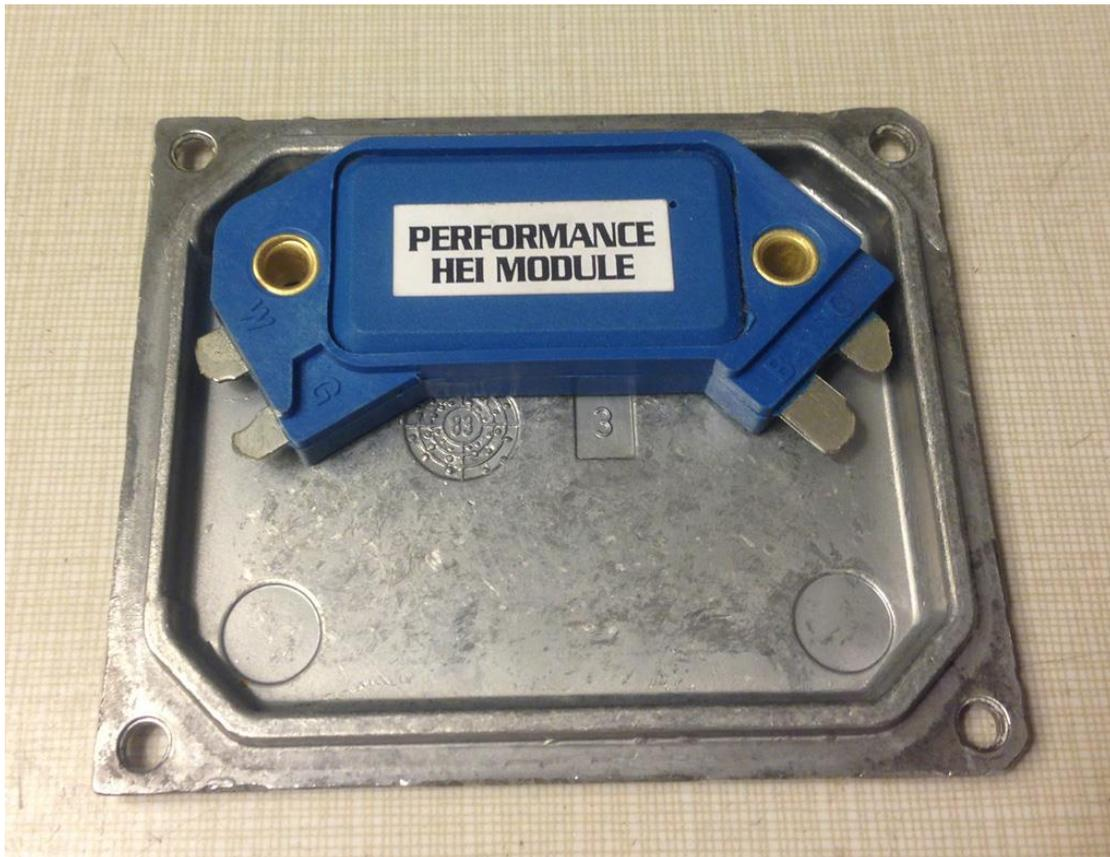
Next, we will mount the module to the cover as shown in the illustration below using the module as a guide.
