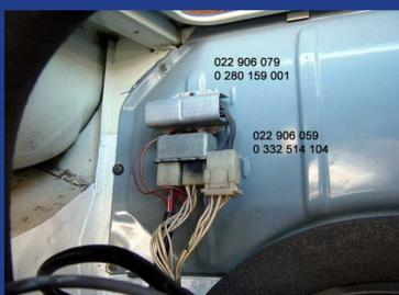
The original relay came in a metal can but has since been replaced by this black plastic version:
