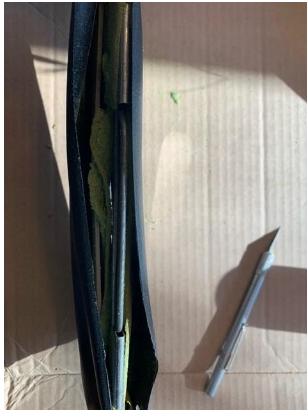
Figure 2 -Edge cut using Exacto knife
