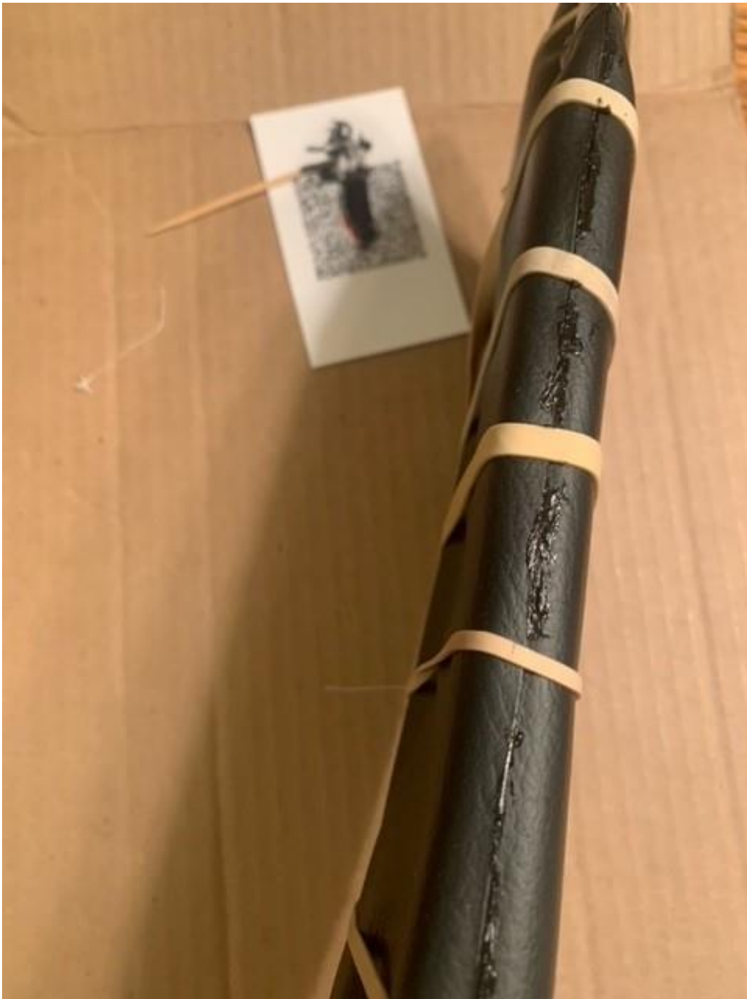
Figure 9 - Black silicon adhesive applied between rubber bands along seam
