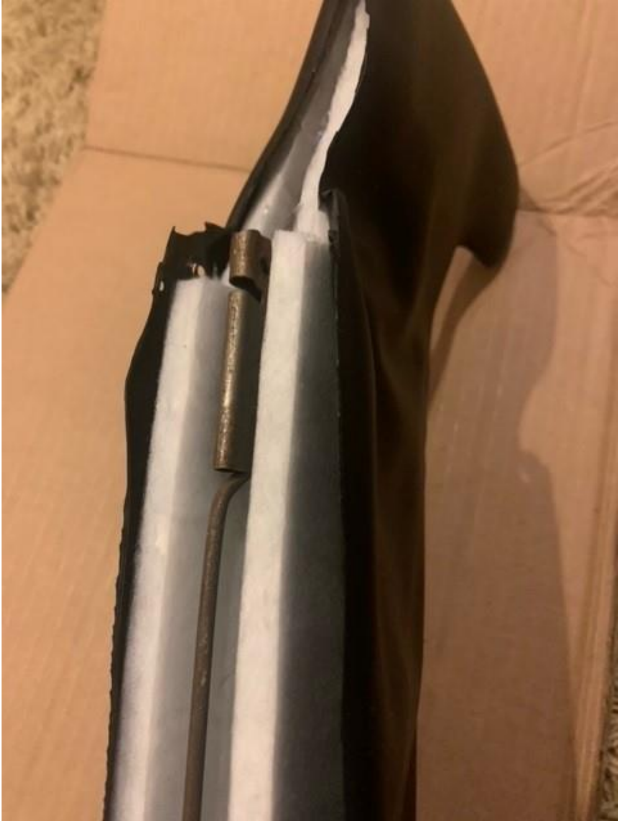
Figure 7 -Foam and Wire Frame in Vinyl
