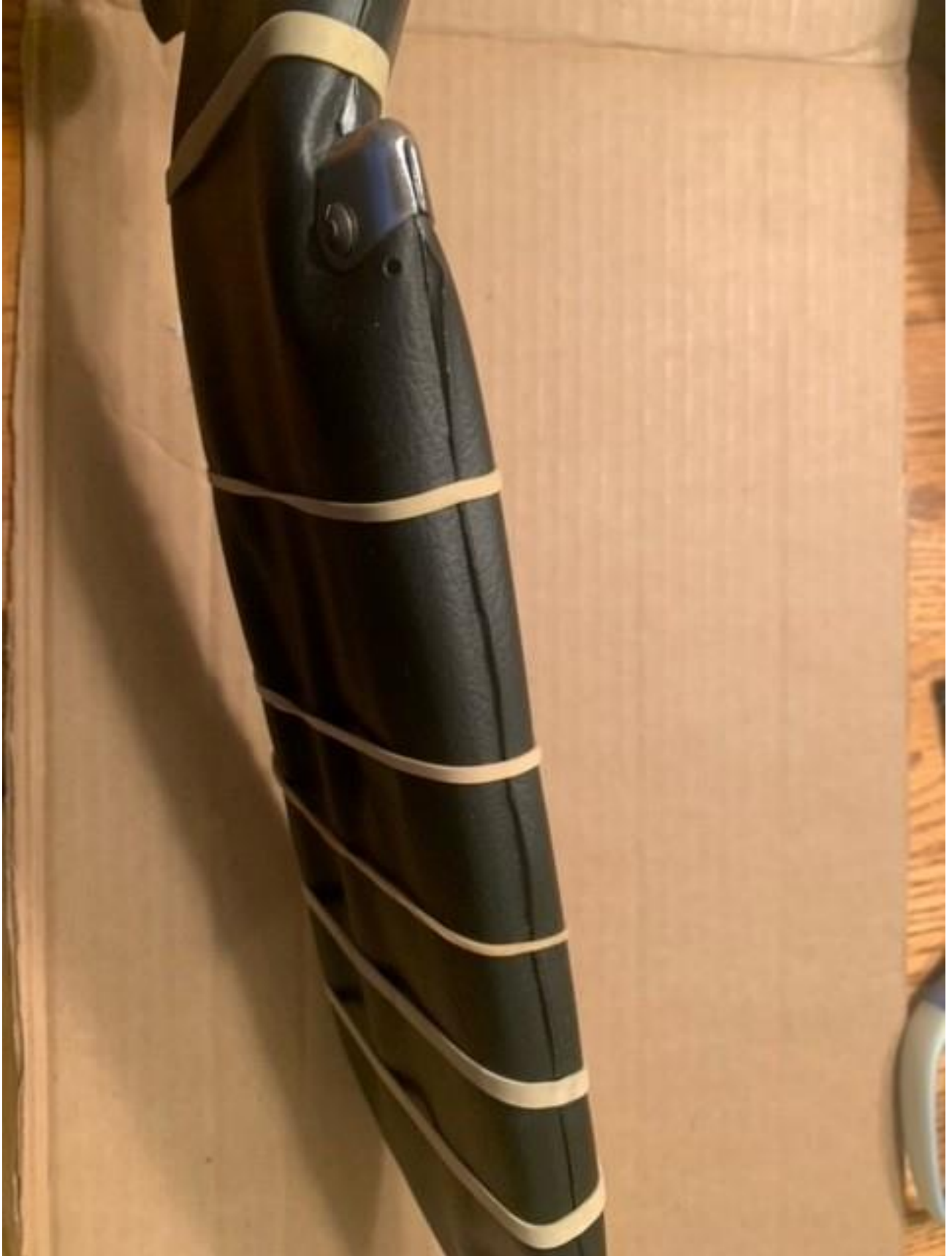
Figure 8 -Rubber bands holding vinyl seam together for gluing
