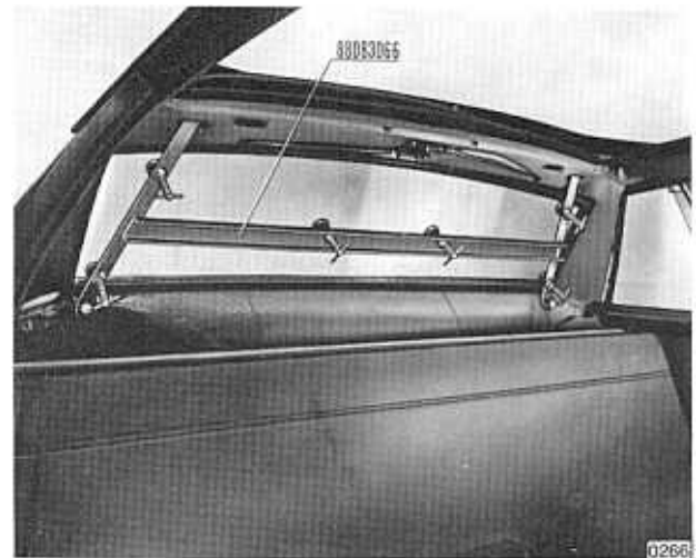
Fig. 15 2/7 - Rear window adhesion fixture.
