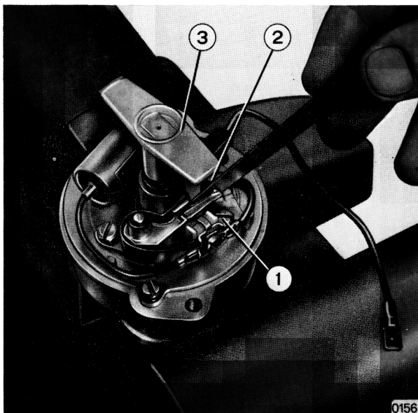
Fig. 01 4/1 - Checking the breaker points.
