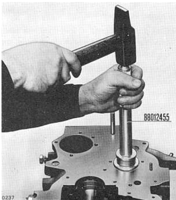
Fig. 01 3/38 - Removing the Ancillary Units Drive Shaft Front Bearing using tool 88012455.
