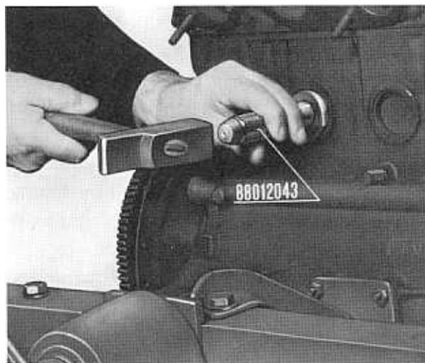
Fig. 01 3/47 - Fitting engine block plug using installing tool 88012043.
