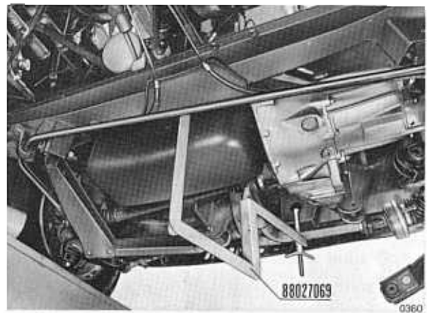
Fig. 03 2/8 - Cradle 88027069 used to support engine.
