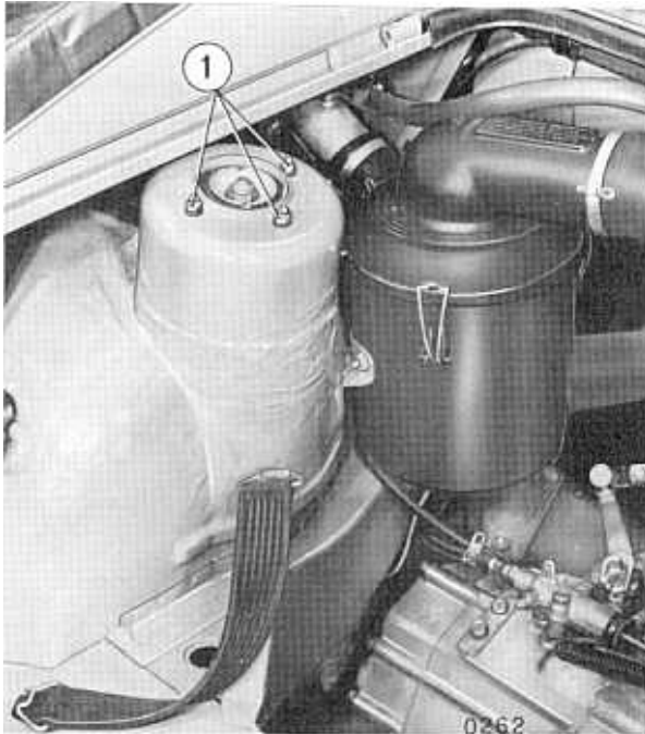
Fig. 07 2/10 - Top view of attachment of strut to body
