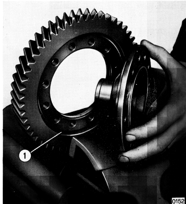
Fig. 03 3/37 - Remounting spur gear on half-casing
