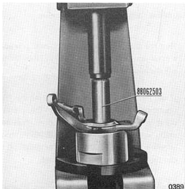
Fig. 08 4/2 - Detachment of bearing from swivel
