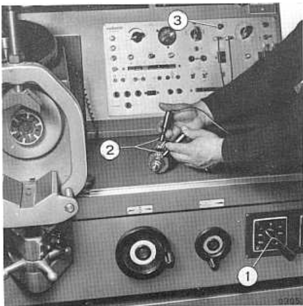
Fig. 14 4/4 - Checking armature insulation
