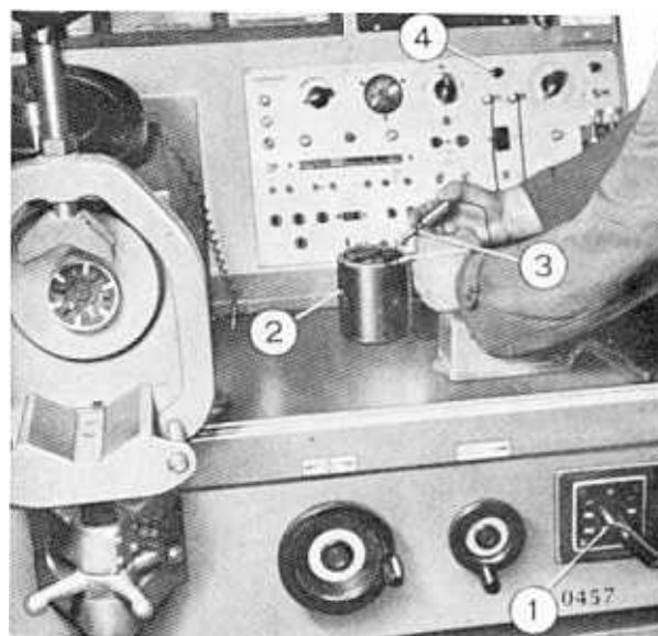
Fig. 14 4/8 - Checking the Field Coils For Continuity
