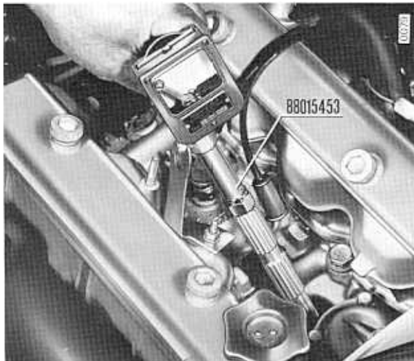
Fig. 01 2/52 - Checking cylinder compressions.
