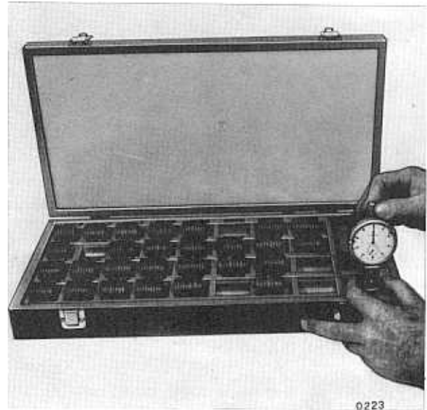
Fig. 01 3/11 - Kit 88013040 consisting of case 88013037, support 88019051 and dial gauge 88095122.
