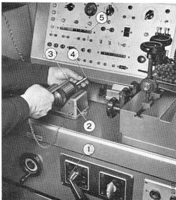
Fig. 14 4/6 - Armature short-circuit check
