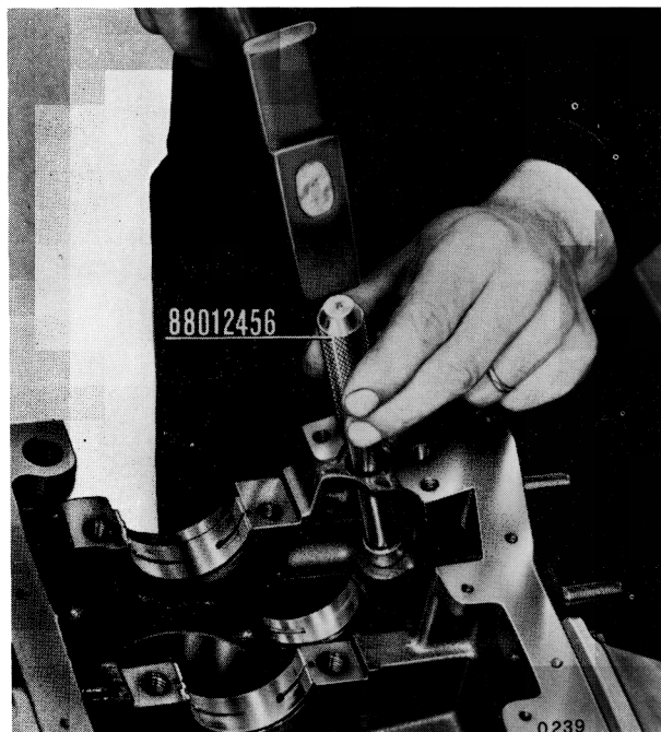
Fig. 01 3/41 - Removing and installing oil pump drive gear bushing.
