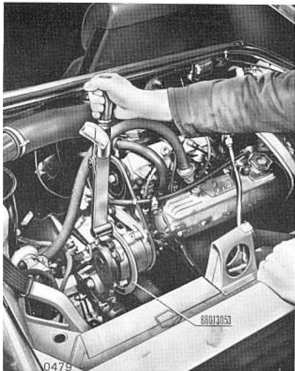
Fig. 01 2/54 - Air pump belt stretcher.
