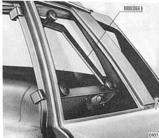
Fig. 15 2/9 - Side window adhesion fixture.
