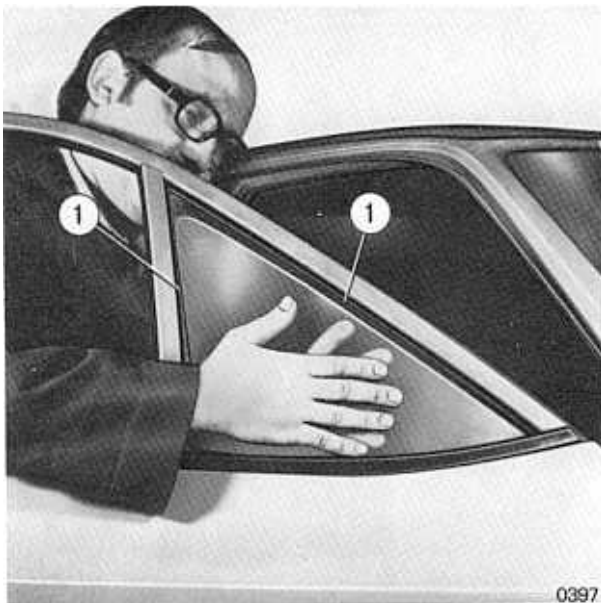
Fig. 15 2/13 - Fitting quarter-light glass.
