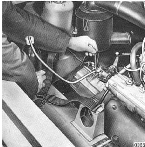
Fig. 02 2/9 - Bleeding the clutch hydraulic circuit
