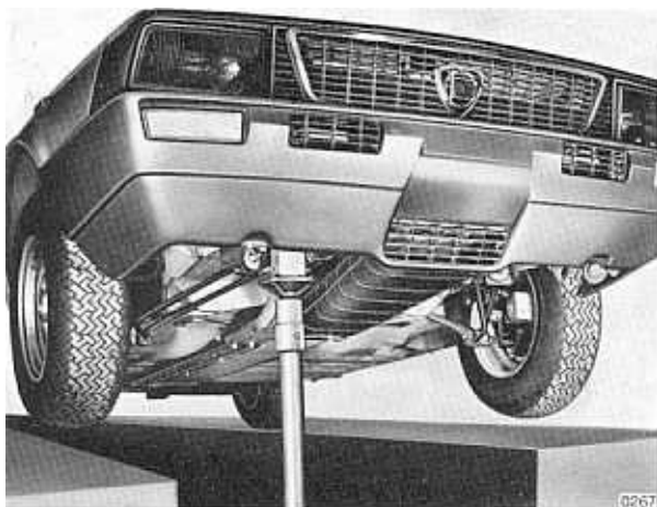
Fig. 07 2/1 - Lifting the car
