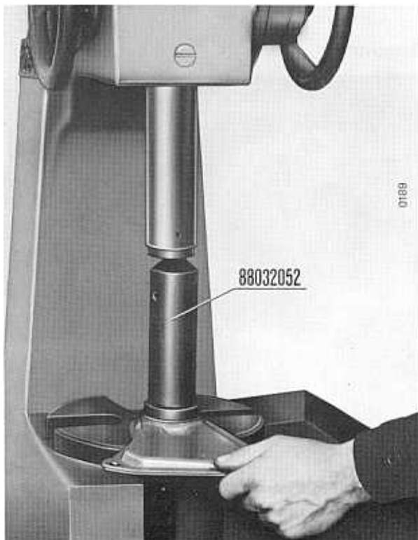
Fig. 01 2/55 - Fixture 88032052 for removing and fitting mounting buffer.
