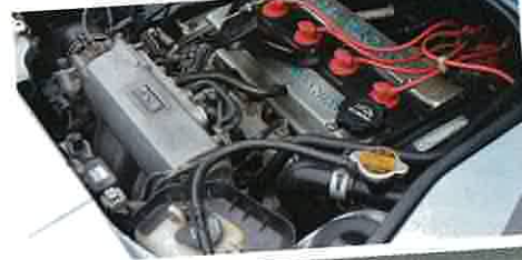
Four-cylinder, 16-valve, twin cam kicks out 123bhp.
